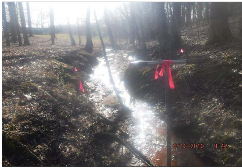
Looking upstream at stream reach 52-E. The reach had severely incised, eroded banks. The right riparian buffer consisted of 90% forest cover with greater than 60% canopy cover and 10% forest with 30-60% canopy cover and maintained understory. The left riparian buffer consisted of 55% forest cover with greater than 60% canopy cover and 45% forest with 30-60% canopy cover and maintained understory. The in-stream habitat was suboptimal with stable features throughout 30-50% of the reach. Channel alterations included a culvert.
