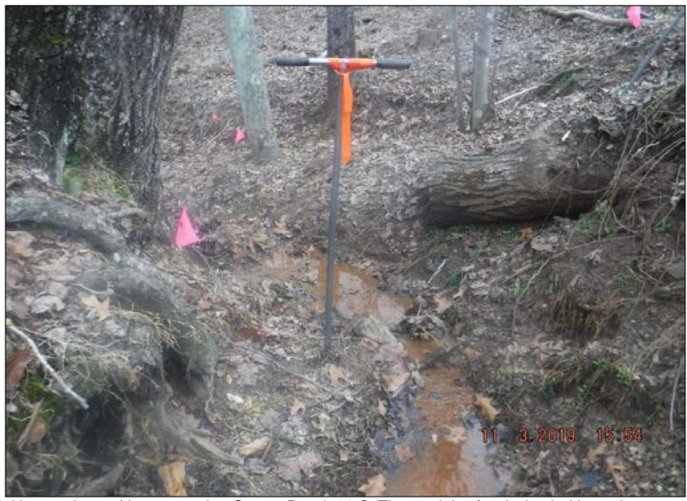
Looking southwest (downstream) at Stream Reach 61-C. The reach is often incised with erosion present on 40-60% of banks. The left bank riparian buffer is heavily encroached upon by impervious surfaces (road) and has some forested areas with 30-60% canopy cover. The right bank riparian buffer is entirely forested and exhibits greater than 60% canopy cover. Habitat elements are unstable and are present in less than 10% of the reach. The reach has been significantly altered (60-80%) by the presence of a culvert and the adjacent road.
