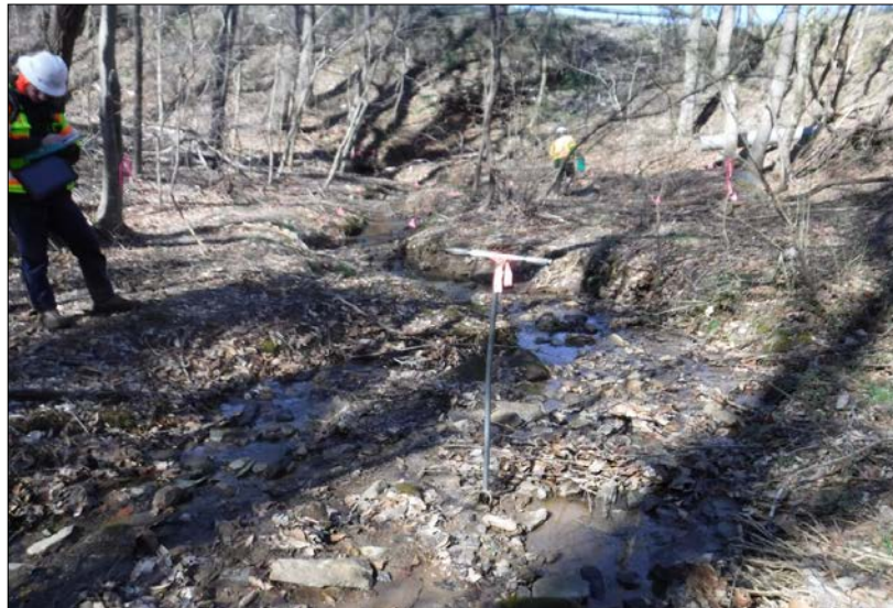
Looking downstream at Reach 13-A. The reach had active erosion in some areas. The right riparian buffer consisted of 40% mature forested areas and 60% impervious surfaces associated with parking lots and roads. The left riparian buffer consisted of 65% mature forested areas and 35% impervious surface associated with parking lots and roads. The in-stream habitat consisted of riffles, pools, leaf packs and substrate of various particle sizes. The stream was degraded by minor amounts of aggregation. The channel was riprapped and channelized through culverts.
