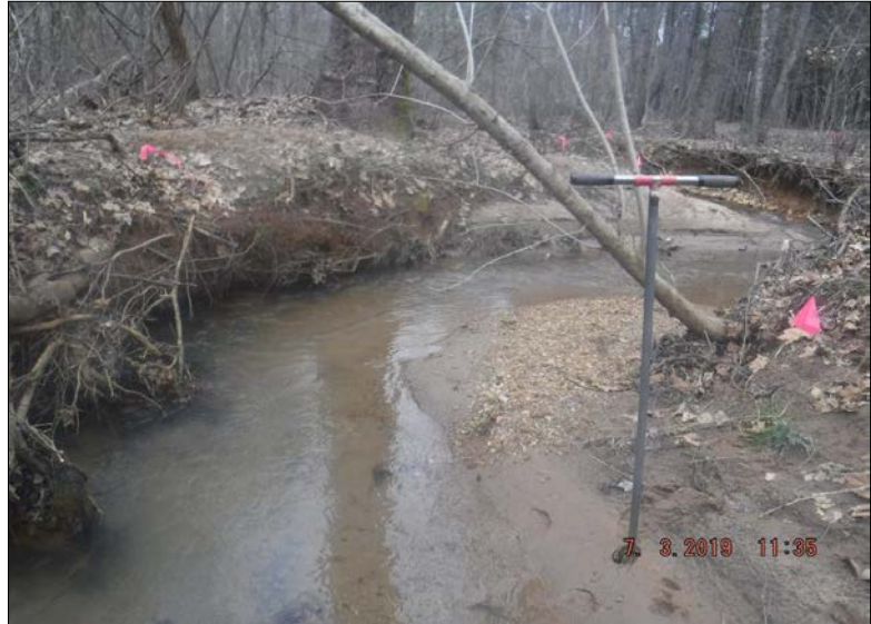
Looking southeast (downstream) at Stream Reach 74-A. The reach exhibits a few incised and/or undercut banks but the majority of the streambank is stable. Both banks' riparian buffers are forested with greater than 60% tree canopy cover. Stable habitat elements are present and occupy 30-50% of the reach. The stream shows no signs of alteration.
