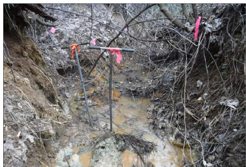
Looking upstream at Reach 17-A. The reach was severely incised with frequent, active erosion throughout. The riparian buffers consisted of 85% mature tree cover and 15% impervious surfaces associated with State Route 220. The in-stream habitat was degraded by severe aggregation. The reach was channelized riprapped at a culvert.
