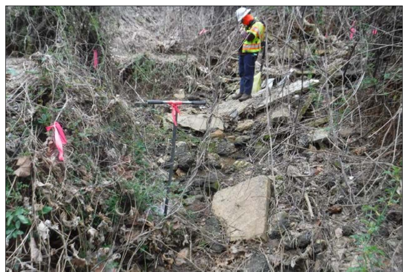
Looking upstream at Stream Reach 14-A. The reach was poor with frequent, active erosion throughout. The right riparian buffer consisted of 45% mature tree cover, 15% non-maintained herbaceous vegetation, and 40% impervious surfaces associated with State Route 220. The left riparian buffer consisted of 55% mature tree cover, 5% non-maintained herbaceous vegetation, and 40% impervious surfaces associated with State Route 220. The in-stream habitat was degraded by severe erosion. The reach was channelized through culverts.
