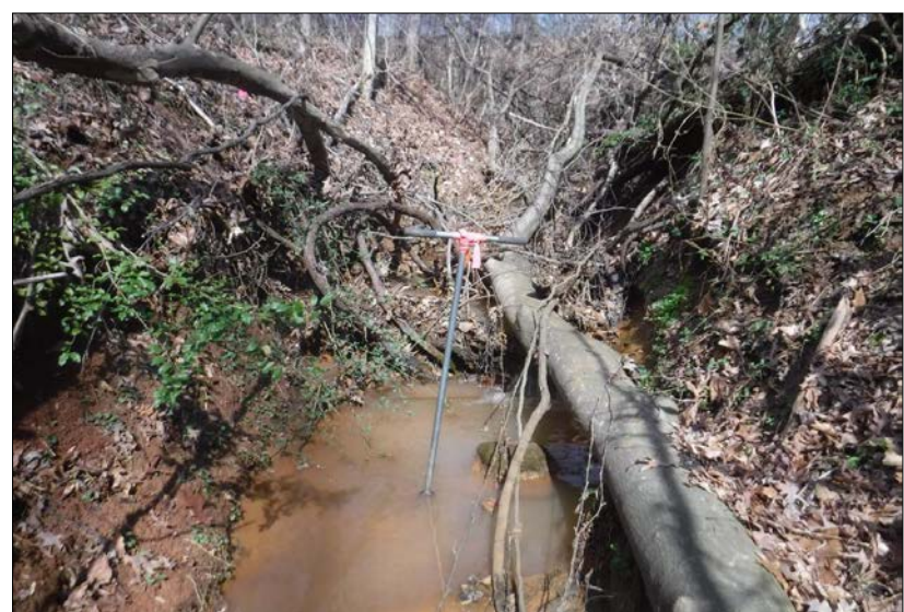
Looking upstream at Reach 7-B. The reach was incised with areas of active erosion throughout and severe aggregation in pools and areas of slow-moving water. The riparian buffers consisted of 60% mature tree cover and 40% impervious surfaces associated with State Route 220. In-stream habitat was present in less than 10% of the reach and was degraded due to severe aggregation. 60-80% of the channel was culverted under State Route 220.
