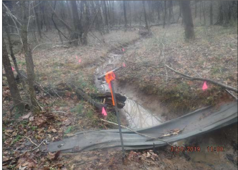
Looking south (downstream) at Stream Reach 70-A. The stream shows signs of erosion but the banks are mostly stable (60-80%). Both banks' riparian buffers are fully forested (>60% canopy cover). Instream habitat elements are present in 10-30% of the reach. The upstream end of the reach is fed by a culvert and rip rap is present immediately below; channel alteration effects 40-60% of the stream reach.
